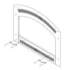
4) Place the emblem over the emblem design on the surround. Insert the studs through the holes. To secure them first put on the split lock washer and then the nut and tighten.
